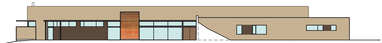
SOUTH AND NORTH ELEVATIONS ■ CONCRETE ■ GLASS ■ STUCCO ■ HARDWOOD SIDING ■ RAMMED EARTH
